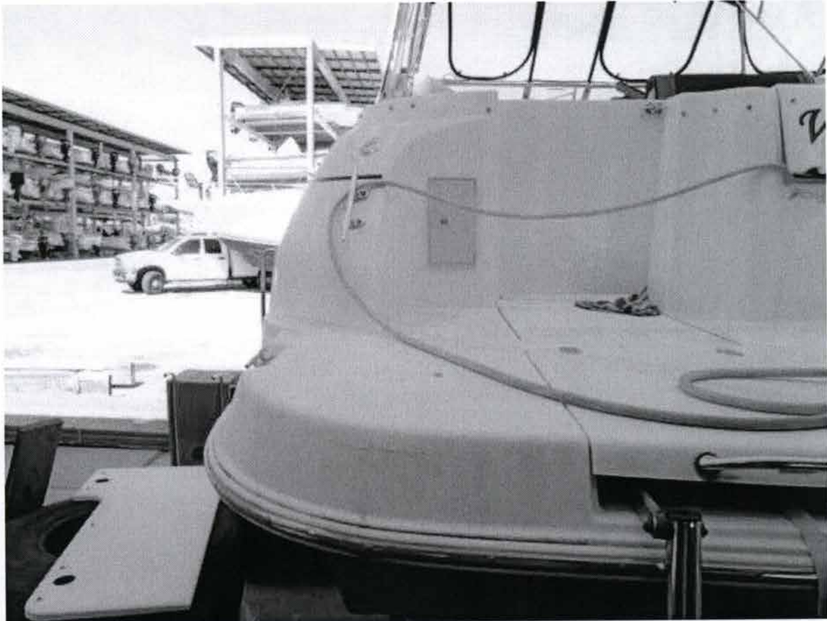
Port side of the swim platform exterior – SS rub rail is pushed down and exterior is cracked – note that exterior does display new & old cracks that can be easily overlooked
