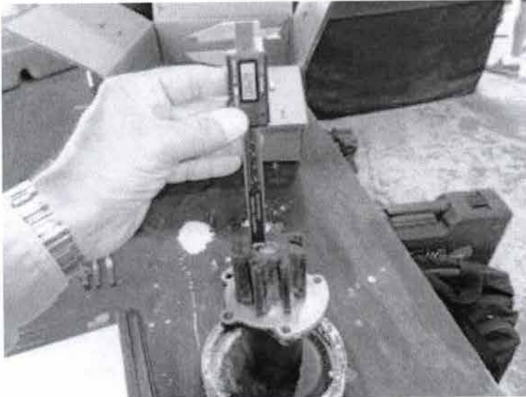
Dial indicator readings of the shaft to the impeller gap
