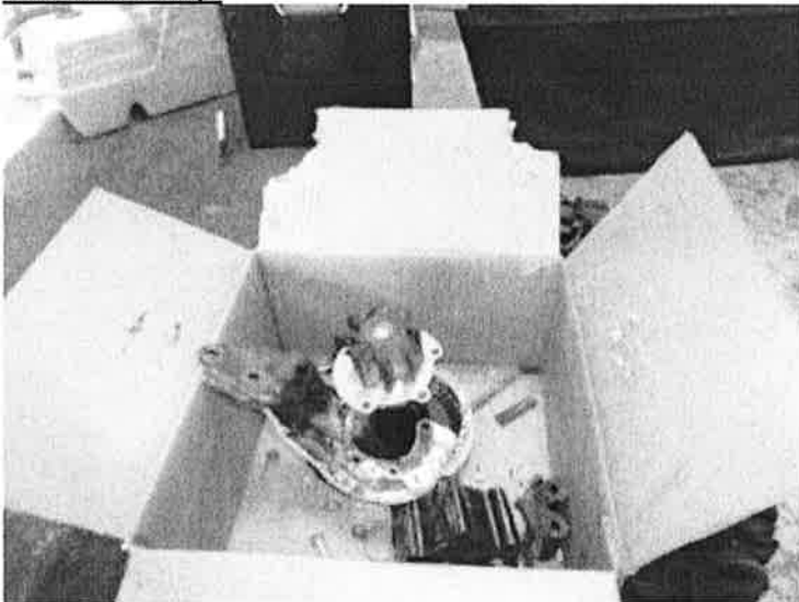
Raw water as produced. Box was not secured and we noted that the O-ring was missing
